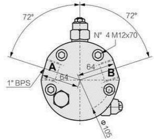
Distributor with double overcentre valve and high pressure pilot line(C)
